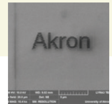
The word "Akron" has been etched onto a sample using Focused Ion Beam technology on NCERCAMP's SEM. At only 10 \mu\text{m} , this etching is about 1/5 the thickness of a human hair.
